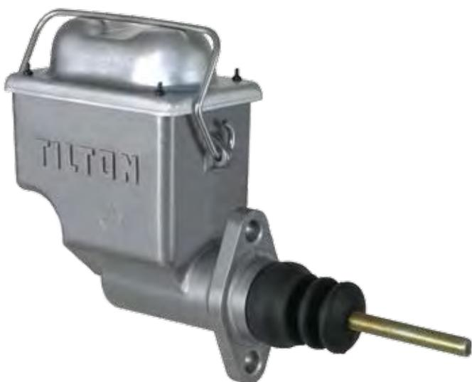
**73**-Series master cylinders are designed for applications that require large fluid capacity in a leak-proof integral reservoir. These cylinders are also unique in that they may be temporarily inverted without loss of fluid. Fluid chamber is completely sealed from the outside environment while still allowing fluid level changes. Available in the most popular bore sizes, these cylinders are an affordable solution for the budget racer.
