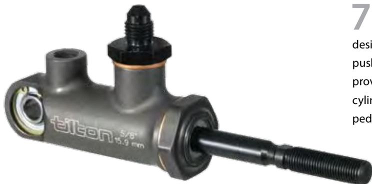
**77**-Series master cylinders offer the latest in racing master cylinder technology in a very lightweight and compact design. The rear spherical bearing mount and one-piece piston/pushrod eliminate side thrust into the master cylinder bore, providing consistent and repeatable braking. 77-Series master cylinders are designed specifically for use with TB&C 900-Series pedal assemblies and balance bars.
