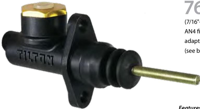
**76**-Series master cylinders share the same compact body design of the 75-Series master cylinders, but feature an AN4 (7/16"-20) inlet port adapter. The inlet port is designed to accept AN4 fittings when remote-mounted reservoirs are used, or the adapter can be removed to accept TB&C billet aluminum reservoirs (see below).
