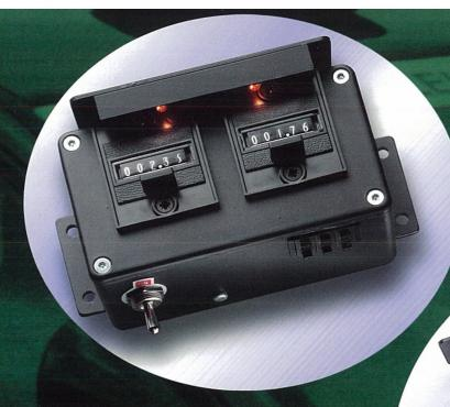
The Retrotrip 2 is designed for historic rallying and carries approval from rally organisers around the world. The two electro-mechanical readouts click over precisely at one hundredth of a mile or km and can be zeroed independently. Calibration is by the three digit selector on the base in the same way as Brantz rally meters. Use any Brantz sensor. Positive or negative ground. The all-metal case is 120mm x70x55.
